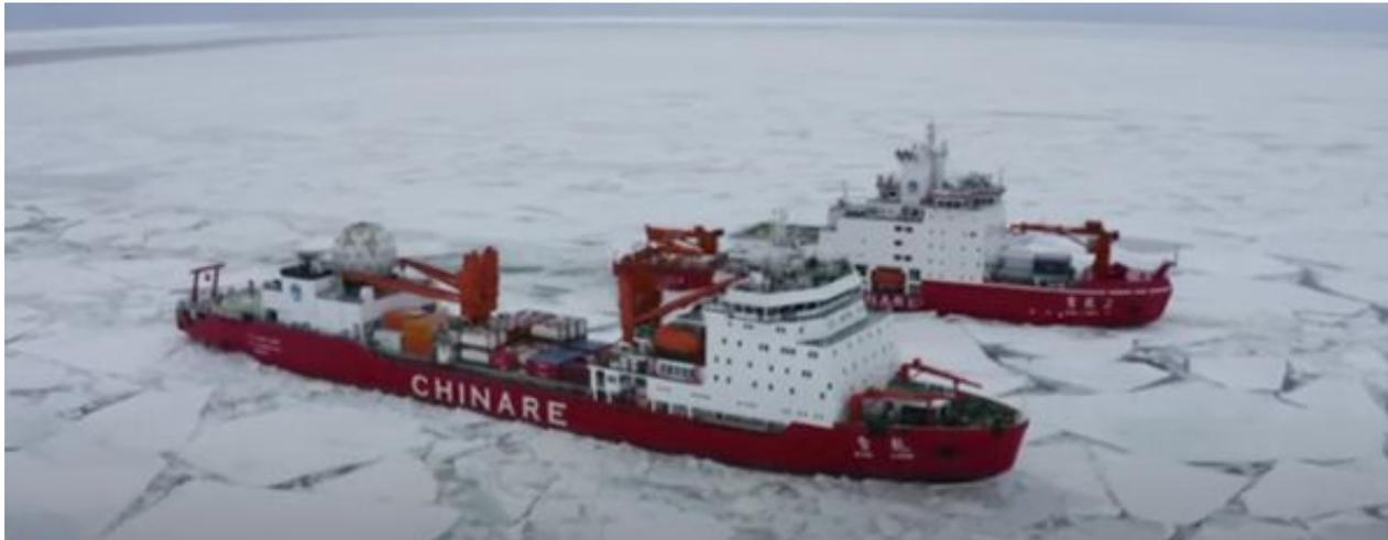
*Image: The newly-commissioned icebreaker Xuelong-2 (accompanied by the first Xuelong) conducts icebreaking test operations during its maiden voyage to Antarctica, November 2019.*
