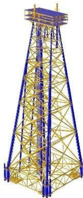
Figure 2: LF15-1 DPP Jacket Design
