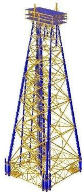
Figure 2: LF15-1 DPP Jacket Design
