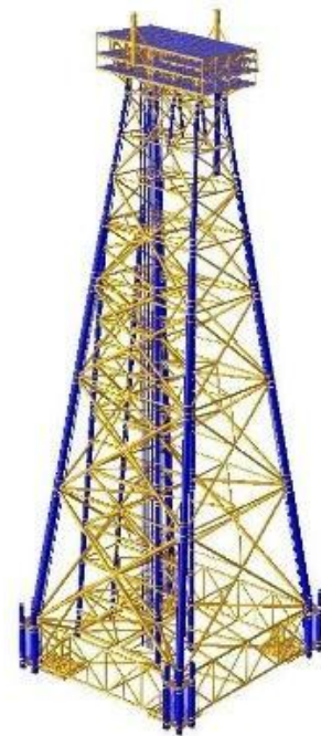
Figure 2: LF15-1 DPP Jacket Design
