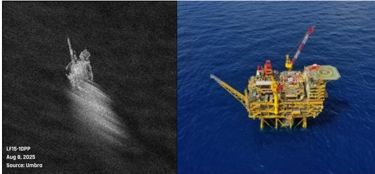
Figure 4: LF15-1DPP Fixed Deepwater Jacket Platform Oil Rig Captured With SAR (Left) and Optical (Right)
